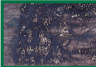
Aluminum Micro-Welding on Piston Ring Side Face
