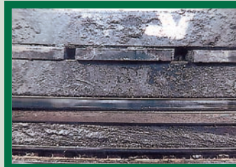
Piston Ring Breakage Caused by Excessive Piston Groove Wear
